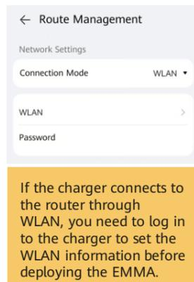
If the charger connects to the router through WLAN, you need to log in to the charger to set the WLAN information before deploying the EMMA.
