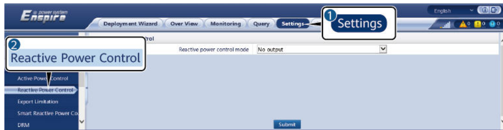
Figure 6-83 Reactive power control
