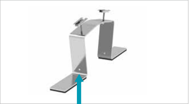
Tighten the grounding wire at the square hole in the Middle Bracket
