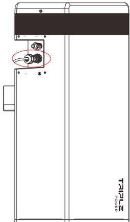
2. Insert the other end of the CAN communication cable to the CAN connector (II) on the first battery which is marked in red. Assemble the cable gland and tighten the cable cap.
