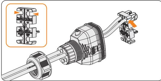
Figure 7-38 Installing RJ45 terminal to the cable fixture
