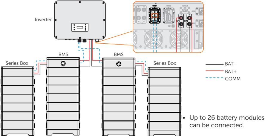
Figure 7-22 Battery connection in two strings (T-BAT-SYS-HV-S2.5/3.6)
