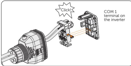
Figure 7-39 Inserting the connector to COM 1
