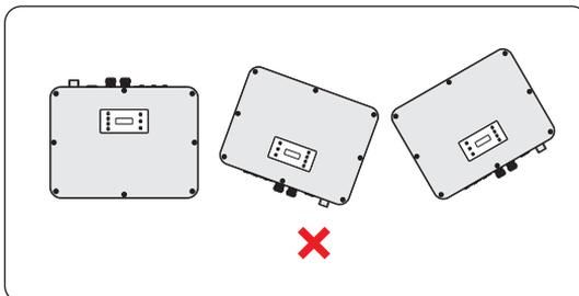
Figure 6-2 Incorrect installation
