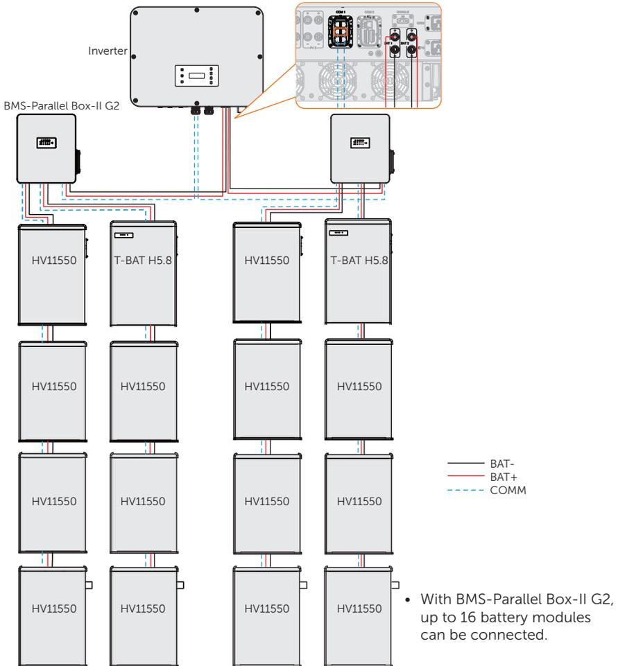
Figure 7-24 Battery connection with BMS-Parallel Box-II G2
