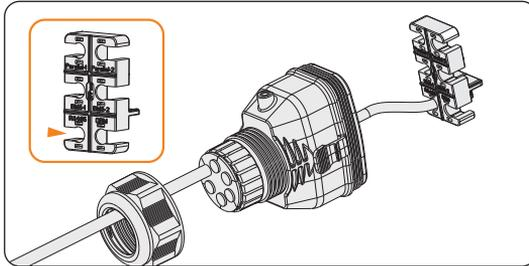
Figure 7-45 Installing RJ45 terminal to the cable fixture
