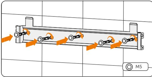
Figure 6-7 Inserting the screws
