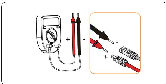
Figure 7-19 Measuring the voltage of PV connectors
