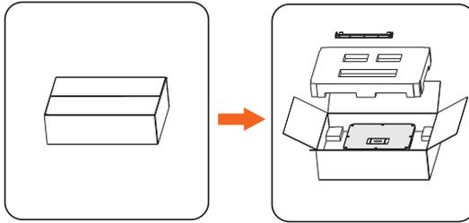
Figure 5-1 Unpacking the inverter
