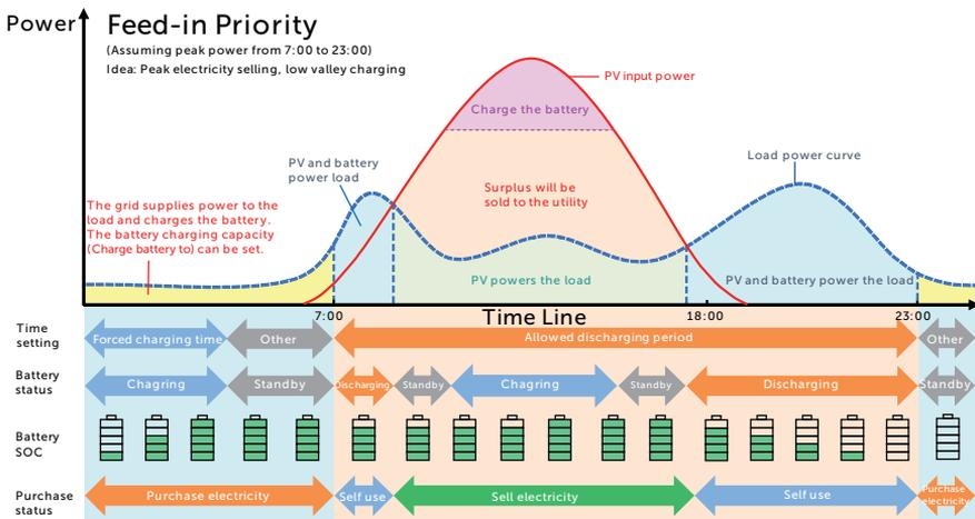
Figure 2-13 Feed-in priority (The grid has limitation)
