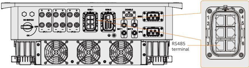
Figure 14-8 Connection terminal for EV-Charger
