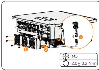
Figure 11-1 Disconnect the fans connectors
