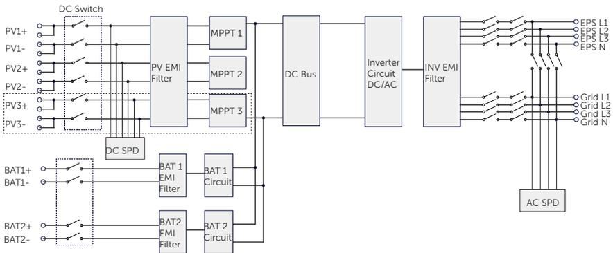
Figure 2-6 Circuit Diagram for X3-ULTRA series inverter
