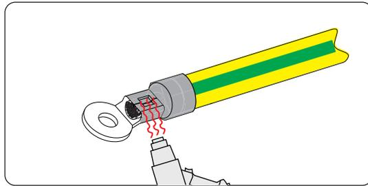
Figure 7-5 shrinking the tubing
