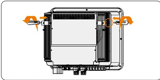
Figure 6-8 Install the Handles
