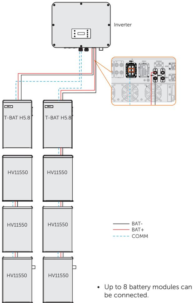
Figure 7-23 Battery connection in two strings (T-BAT-SYS-HV-5.8)
