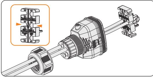
Figure 7-42 Installing RJ45 terminal to the cable fixture
