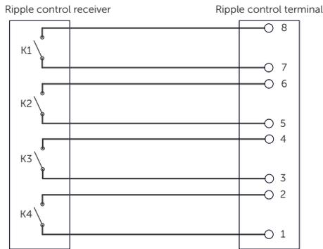
Figure 7-56 Connection diagram for ripple control
