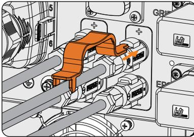
Figure 12-4 Removing the Battery connector
