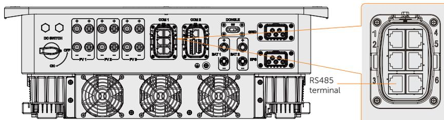
Figure 14-11 Connecting terminal for Datahub
