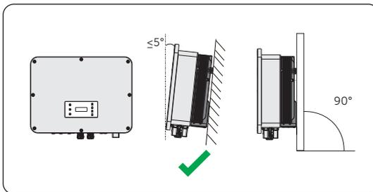
Figure 6-1 Correct installation
