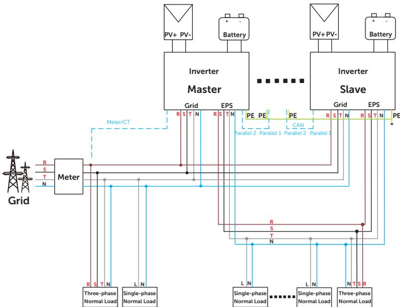
Figure 7-32 System diagram without SolaX X3-PBOX-150kW-G2
