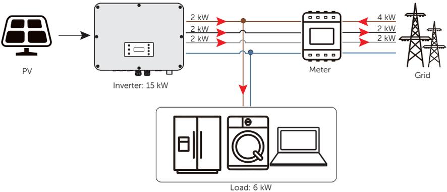
Figure 2-17 Zero export control with **Phase Unbalance** disabled
