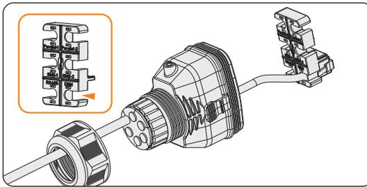
Figure 7-46 Installing RJ45 terminal to the cable fixture
