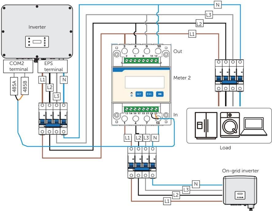
Figure 14-16 Connection diagram of Meter on EPS terminal
