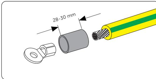
Figure 7-3 Installing the tubing and OT terminal
