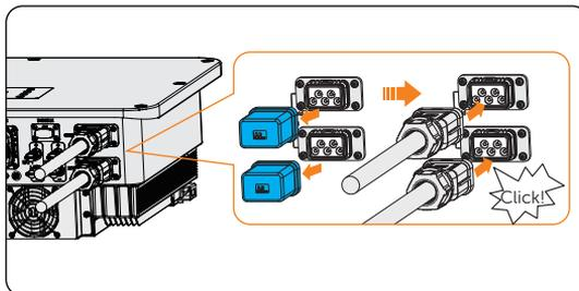
Figure 7-13 Installing the AC connector to inverter
