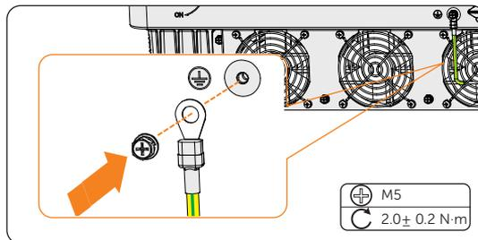
Figure 7-7 Securing the PE cable
